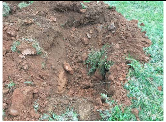
Photo 2 – TP-2 – Rock cobbles encountered in the top 1 foot of the test pit
