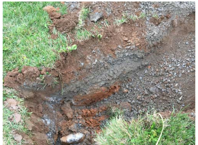
Photo 12 – TP-7 – Soil and apparent CR6 material underlain by natural soils
