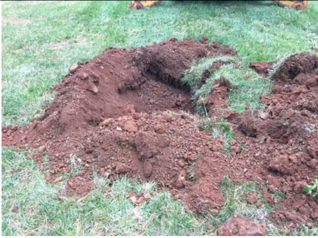
Photo 1 – TP-1 – Showing natural soils at the ground surface
