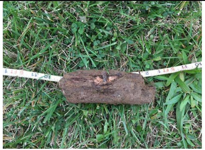
Photo 14 – TP-9 – Organic material (piece of wood) encountered in test pit
