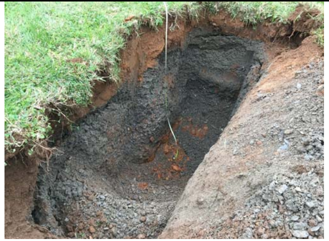
Photo 8 – TP-3 – End of test pit showing apparent CR6 underlain by natural soils
