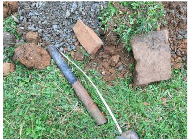
Photo 6 – TP-3 – Pipe (approximately 2 feet in length), brick and concrete material encountered in test pit
