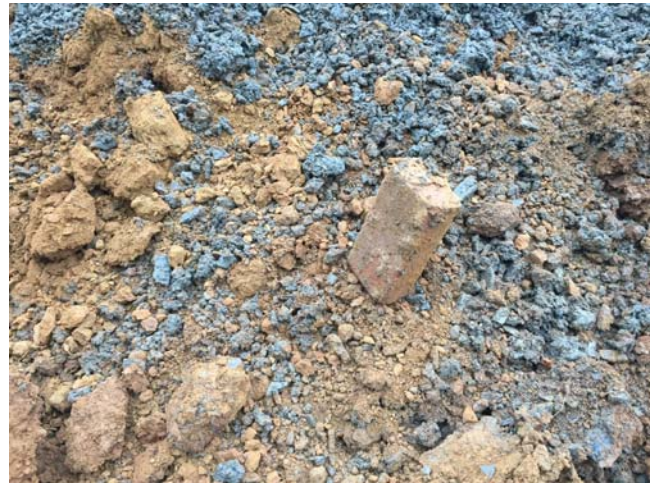
Photo 16 – TP-10 – Brick encountered in the test pit
