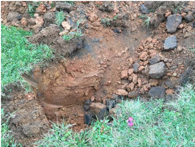
Photo 9 – TP-4 – Asphalt material underlain by natural soils
