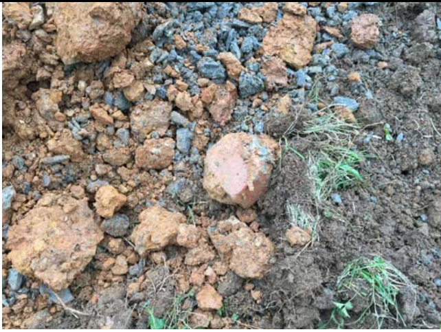
Photo 19 – TP-11 – Brick material encountered in the test pit
