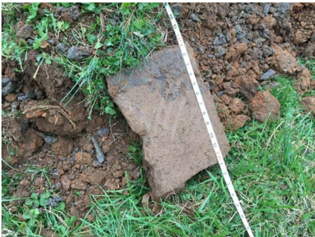
Photo 5 – TP-3 – Concrete material measuring approximately 1'x8"x4" encountered in test pit
