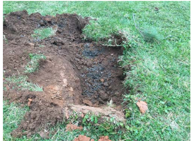
Photo 4 – TP-3 – Beginning of excavation and exposing of apparent CR6 material
