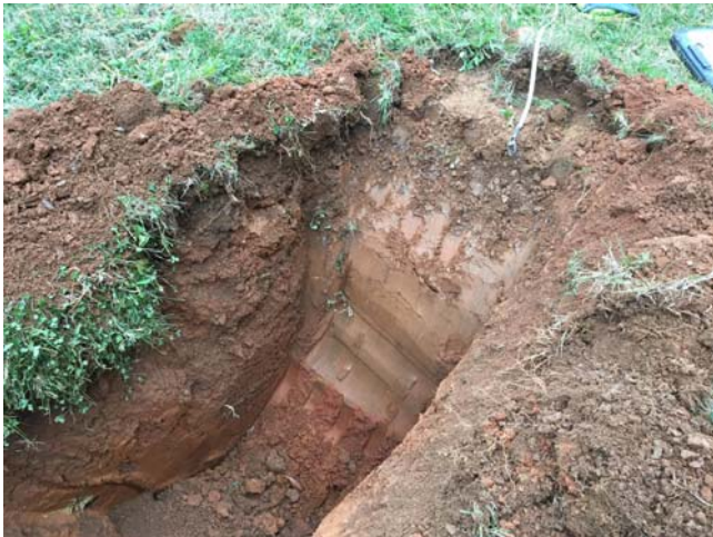
Photo 3 – TP-2 – Showing 2 feet of fill material underlain by natural soils
