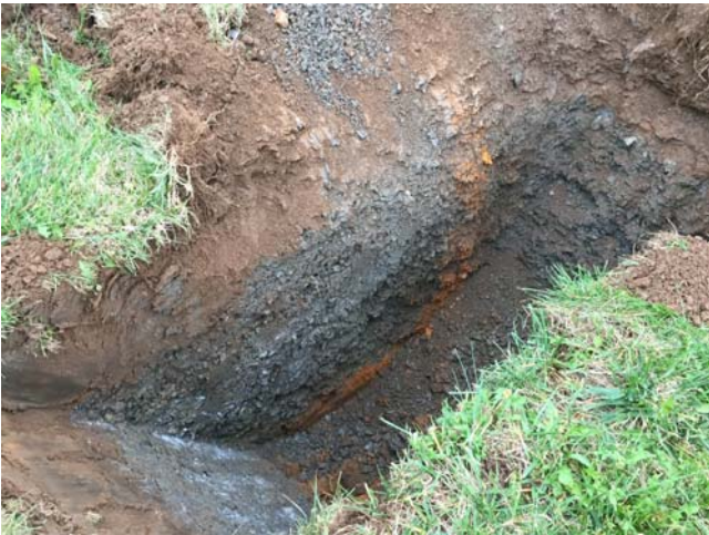
Photo 15 – TP-9 – Apparent CR6 material underlain by natural soils
