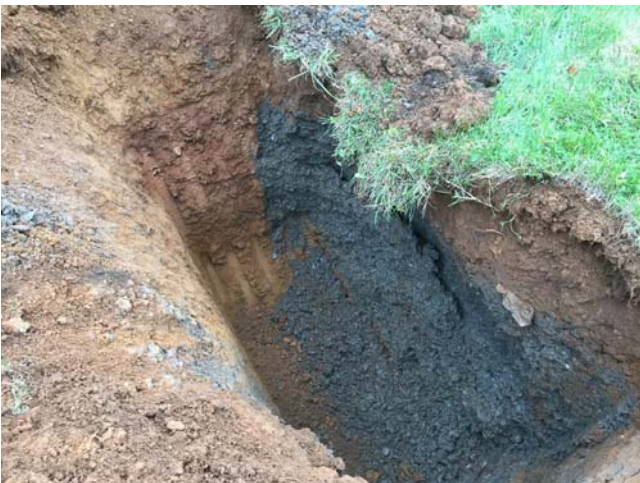
Photo 17 – TP-10 – Apparent edge of fill material showing vertical cut filled with CR6
