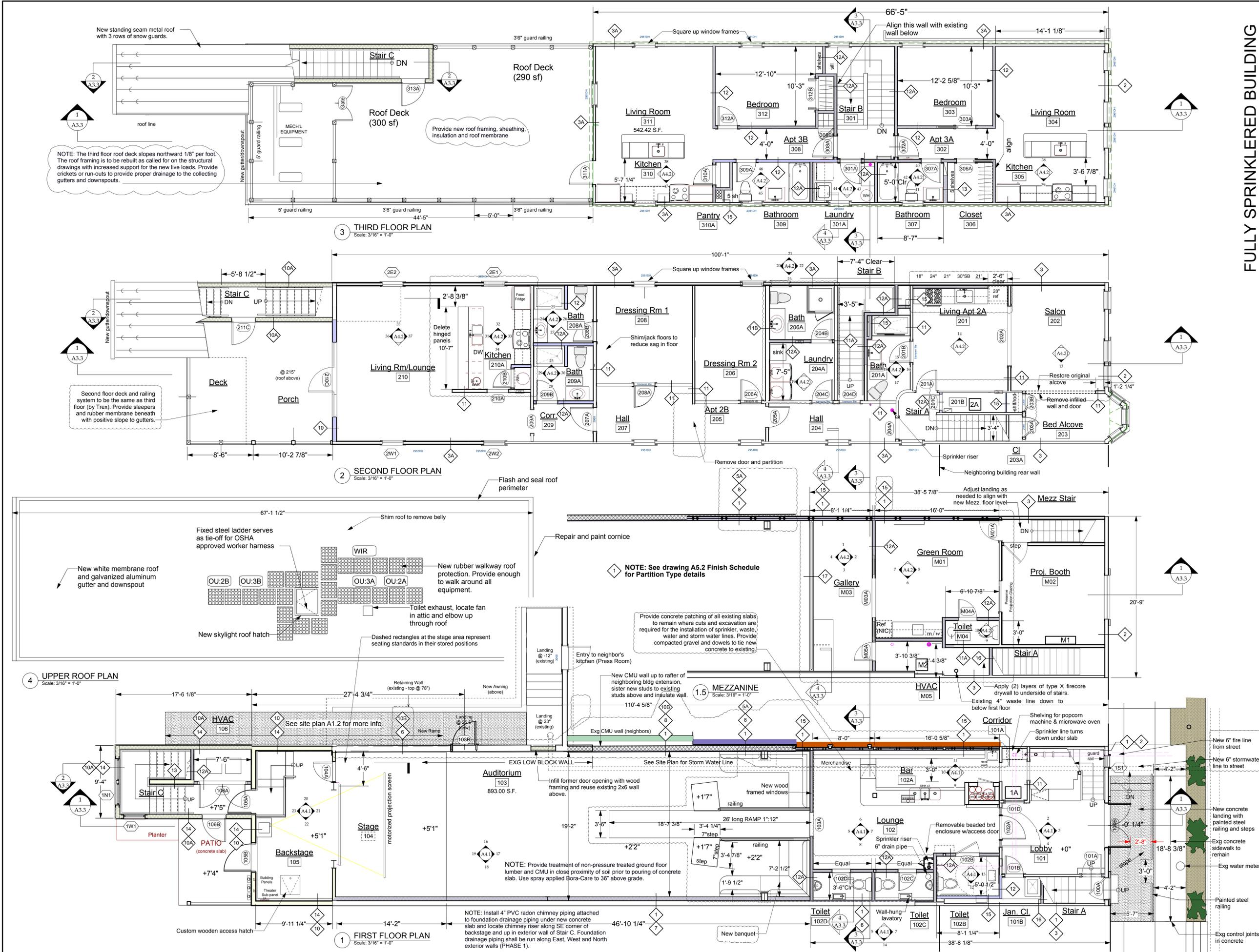
NOTE: The third floor roof deck slopes northward 1/8" per foot. The roof framing is to be rebuilt as called for on the structural drawings with increased support for the new live loads. Provide crickets or run-outs to provide proper drainage to the collecting gutters and downspouts.
