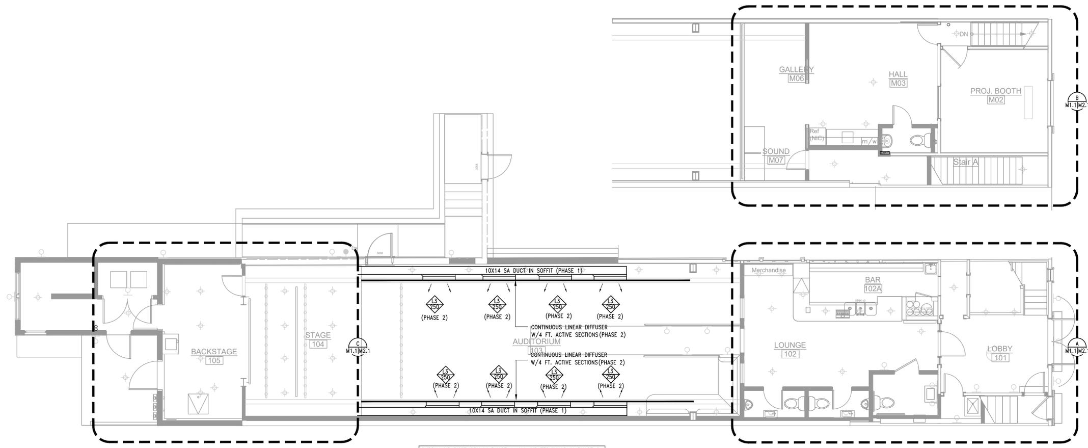
SUPPLY AIR DUCTWORK IN PHASE 1; ALL AIR TERMINALS IN PHASE 2
